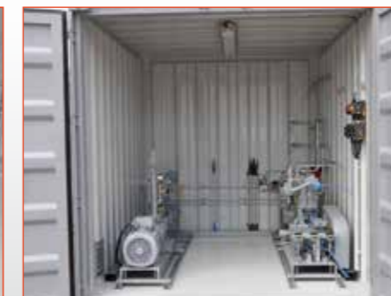
▶ Container version of a pump and compressor system according to customer specification.
