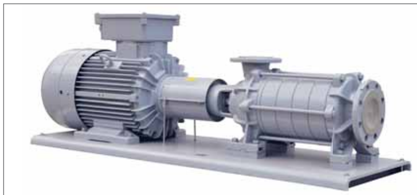
Horizontal, self-priming pump unit in a link-body version with open impellers
