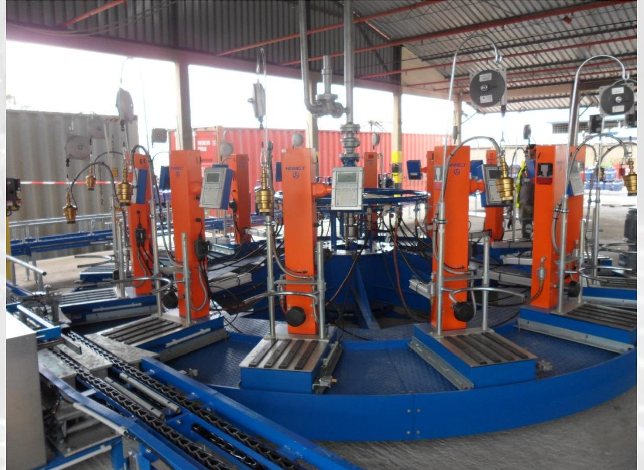
*Carousel Filling Plant K18E with electronic filling scale type WAER*
