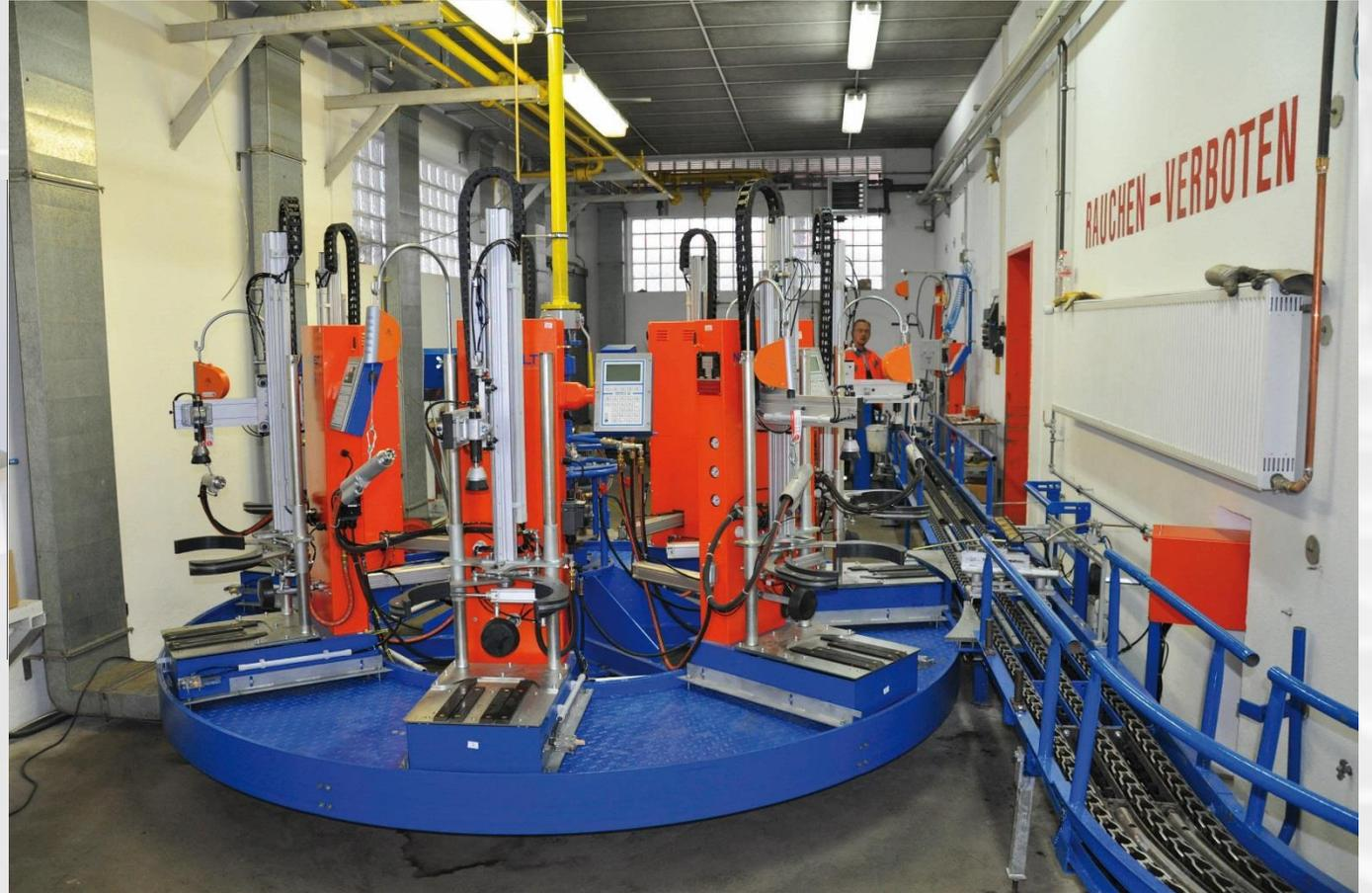
*Carousel Filling Plant K7E with electronic filling scale type WAER*
