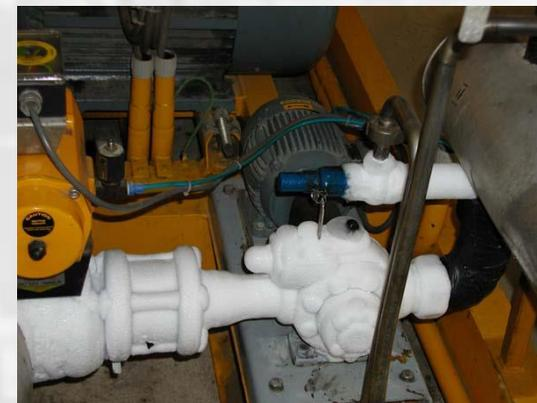
*Hose reels for fire protection, automatic filter for colour, rotary vane pumps for CO2*
