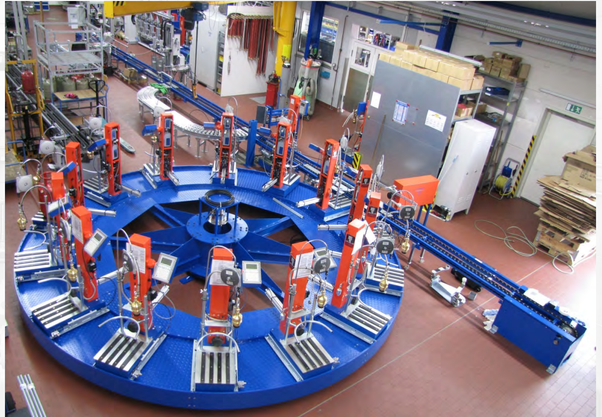
Carousel Filling Plant K18E with electronic filling scale type WAER
