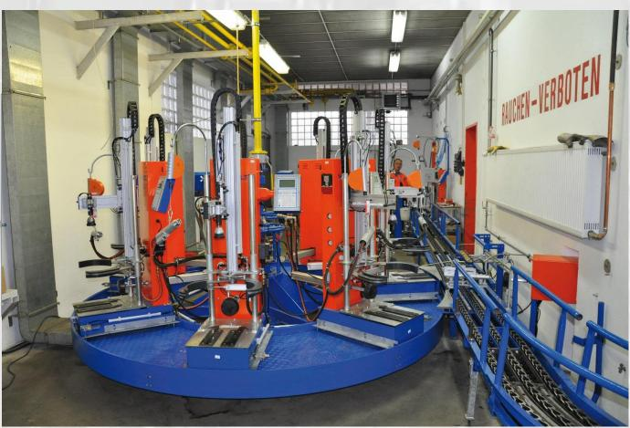
Carousel Filling Plant K7E with electronic filling scale type WAER
