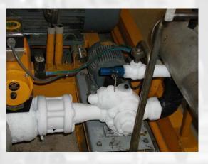
Hose reels for fire protection, automatic filter for colour, rotary vane pumps for CO2
