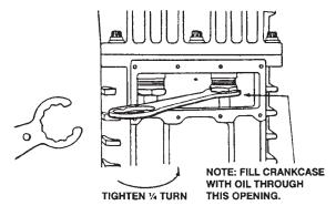
Figure 5.5A: Packing Adjusting Nuts
