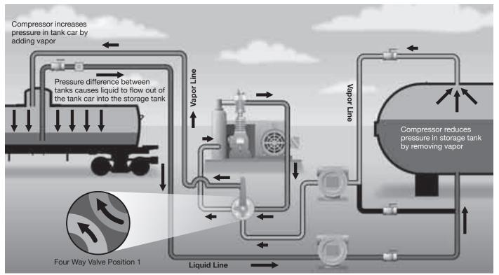
Figure 1.1B: Liquid transfer by vapor differential pressure
