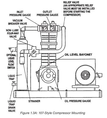
Corken gas compressors are mounted on oil lubricated crankcases that remain at atmospheric pressure. Crankshafts are supported by heavy-duty roller bearings and the connecting rods ride the crankshaft on journal bearings. With the exception of the small size model 91 compressor, all compressor crankcases are lubricated by an automotive type oil pressure system. An automatically reversible gear type oil pump circulates oil through
