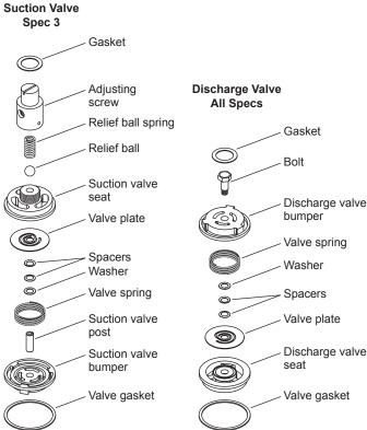
Figure 1.3D: Suction and Discharge Valves
