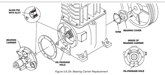
present, the roller bearings should be replaced. When replacing roller bearings, always replace the entire bearing, not just the cup or the cone.
