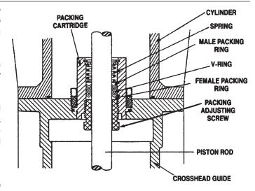
Figure 1.3C: Compressor Sealing System
