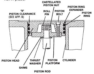
Figure 5.4A: Piston Cross Section Model Sizes 91 Through 491
