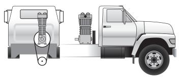
Figure 2.8D: Top Transport Mounting
