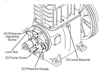
Figure 3.3A: Oil Pressure Adjustment
