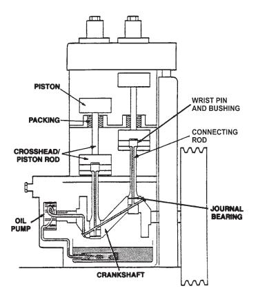
Figure 1.3B: Pressure Lubrication System (Not Available on Model 91)
