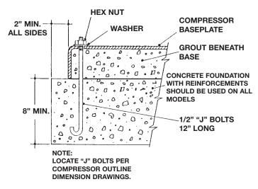
Figure 2.2A: Recommended Foundation Details for Corken Compressors 91 - 691
