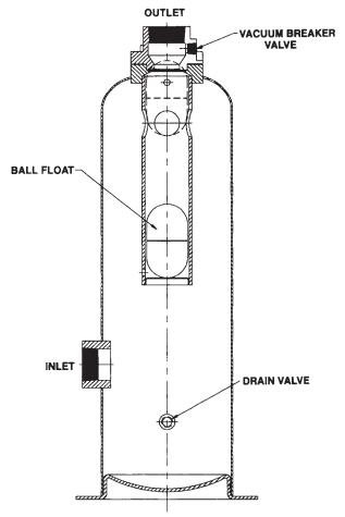
Figure 2.4A: Mechanical Trap
