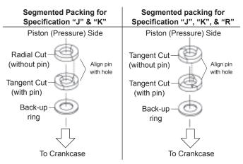
IMPORTANT: Identify and line up the rings before installing. Be sure they face the way shown here and that the pin and hole are aligned when assembled.
