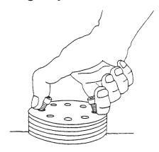
Figure 5.3A: Piston Removal
