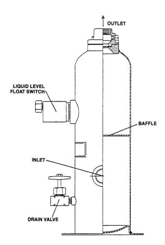
Figure 2.4B: Automatic Liquid Trap
