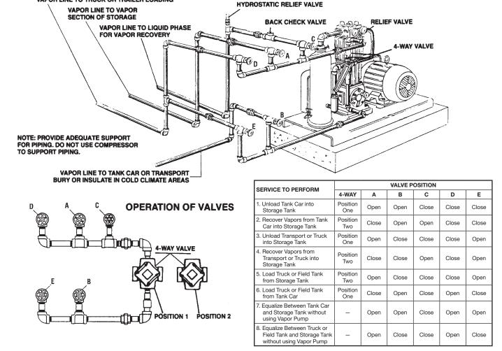
Figure 2.3B: Five-Valve Manifold Piping System
