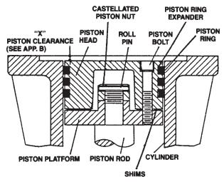
Figure 5.4B: Piston Cross Section Model 691
