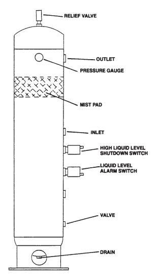
Figure 2.4C: ASME Automatic Liquid Trap
