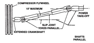
Figure 2.8B: U-joint Drive for Compressor
