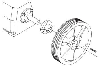
Figure 3.2A: Flywheel Installation
