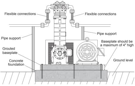
Figure 2.3A: On –107 mountings, the flexible connectors should be located near the four way valve.
