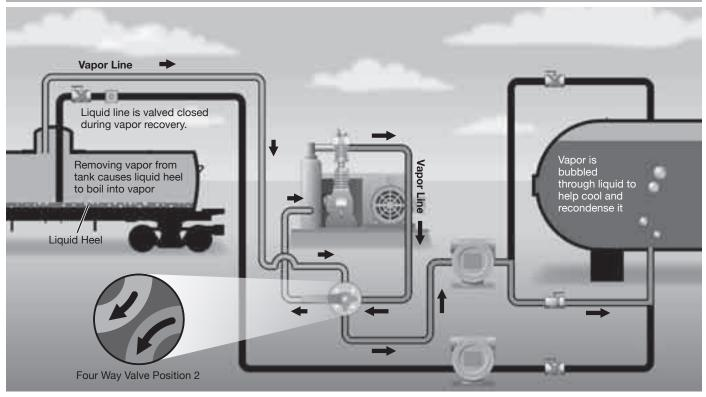
Figure 1.2A: Residual Vapor Recovery
