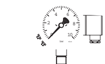
Pressure Gauge with Measuring Transformer
